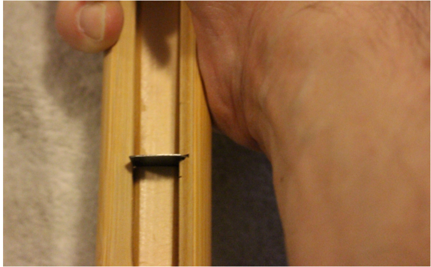
Figure 94: Line up the new slats with the old and squeeze them against the square.
