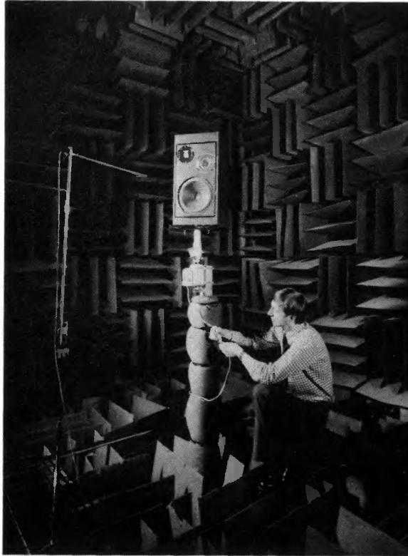
Figure 8.11 Anechoic chamber (courtesy Acoustic Research)
